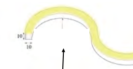
Minimum Bending Radius: 60mm
