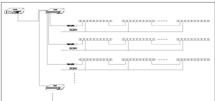
Note: The wire connection must use a waterproof junction box with an IP65 or higher rating. The waterproof joints of the junction box must match the leads of the lighting fixtures. It is recommended that each DMA signal amplifier carry no more than 32 lighting fixtures.
