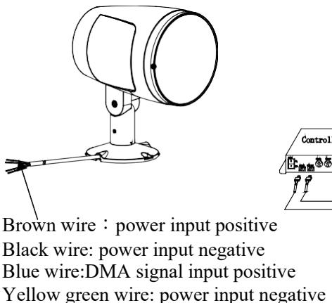
3. Connect each core wire of the lamp to the power input (24V/DC) separately Match and connect the signal input line
