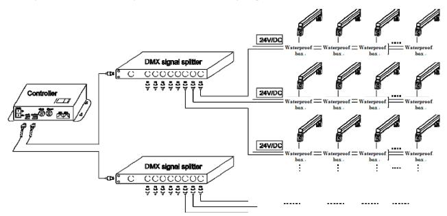
**Note:** The wire connection must use a waterproof junction box with an IP65 or higher rating, and the waterproof joints of the junction box must match the leads of the lighting fixtures. It is recommended that the total length of the splicing of the lighting fixtures connected to each power circuit should not exceed 14 meters, and it is advisable to have no more than 32 lighting fixtures carried by each DMA signal amplifier.
