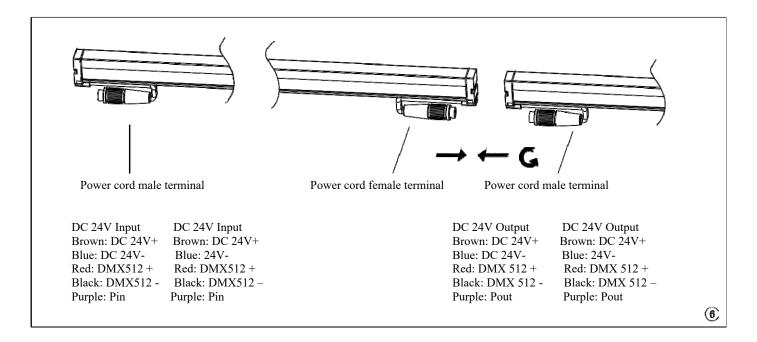
5. Refer to the schematic diagram below for wiring of the lighting fixtures
