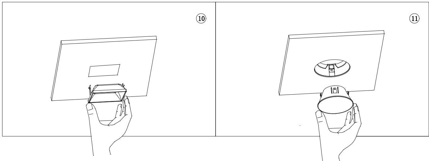
2. The lighting fixture can be adjusted 360 degrees horizontally and 0-21 degrees vertically. The angle needs to be adjusted before installing the reflector cover
