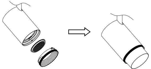
**Note:** When replacing accessories, the spotlight and honeycomb can be installed simultaneously.
