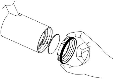
As shown in the above figure, rotate the front cover clockwise by hand until it stops rotating. Then, remove the front cover from the lamp by hand and remove the glass accessories to install the new glass into the lamp.
