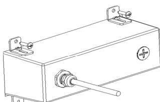
6. The module is connected to the installed lamp body, with the live wire connected to the live wire, the neutral wire connected to the neutral wire, and the ground wire connected to the ground wire.
