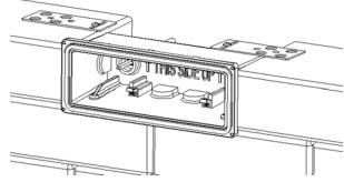
7. Insert the module into the lamp body, install the surface cover, and complete the installation.
