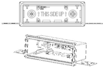
4. Insert the lamp body into the position of a standard brick, use mud to stabilize the position of the lamp body at the porous plate, keep the lamp body level with the wall, and ensure that the distance L between the rear side of the lamp body protrusion and the last wall is  $\geq 0$  (as shown in the right figure below), to avoid contact between the front cover and the wall during subsequent installation.
