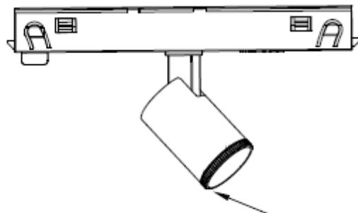
Rotate the front frame to adjust the spot size
