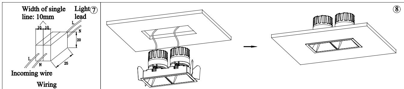
4. Hold the lamp with both hands and insert it into the ceiling hole until the lamp panel is flush with the surface of the ceiling, as shown in Figure⑧⑨⑩.
