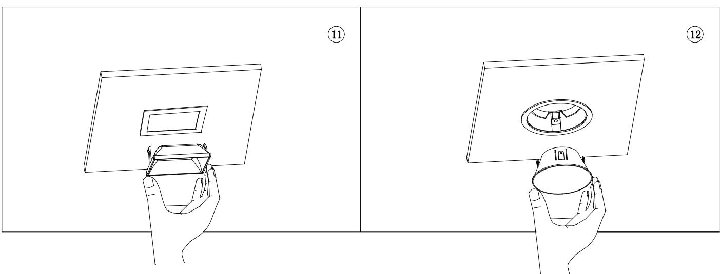
2. The lighting fixture can be adjusted 360 degrees horizontally and 0-21 degrees vertically. The angle needs to be adjusted before installing the reflector cover
